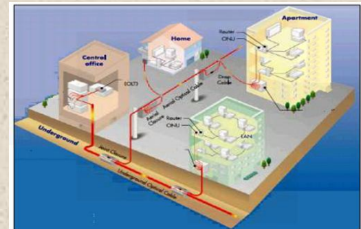
Figure. 33 FTTx - Construction Methodology
